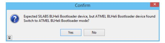
The same will happen if the first automatic "Check" finds Atmel instead of SiLabs or vice versa. (The 4way-interface in SiLabs C2 mode does not provide this kind of automatic detection.)
