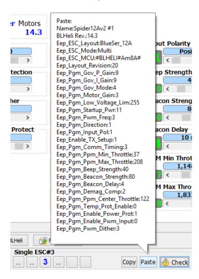
Hovering the mouse over the button shows the current clipboard content to paste. (*ESC # - Name* is never considered in the paste action. *Motor Direction* and *PPM Min/Center/Max Throttle* are only considered if the sync option is turned on).
